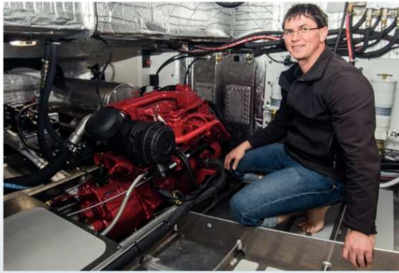
Jason Dickey next to the 90hp engine which powers this 14-tonne displacement vessel at up to 9.5 knots.
